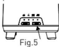
6. Press the "LIGHT" button, to adjust the light mode and intensity - Strong light(default)/weak light/breathing light.
