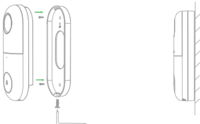
1. Fix the bracket on the wall using the mounting screws
