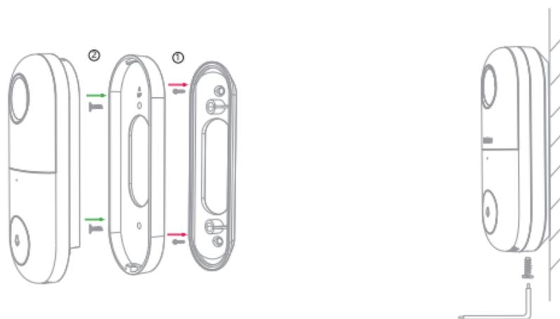
1. Fix the angle wall mount on the wall
